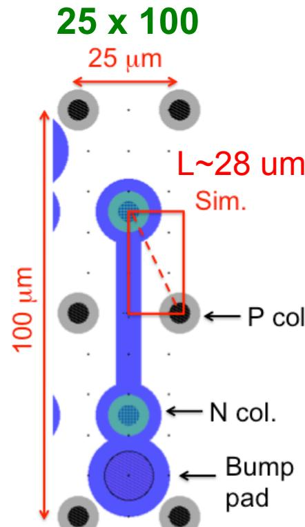
All designs assuming a column diameter of 5  $\mu\text{m}$
