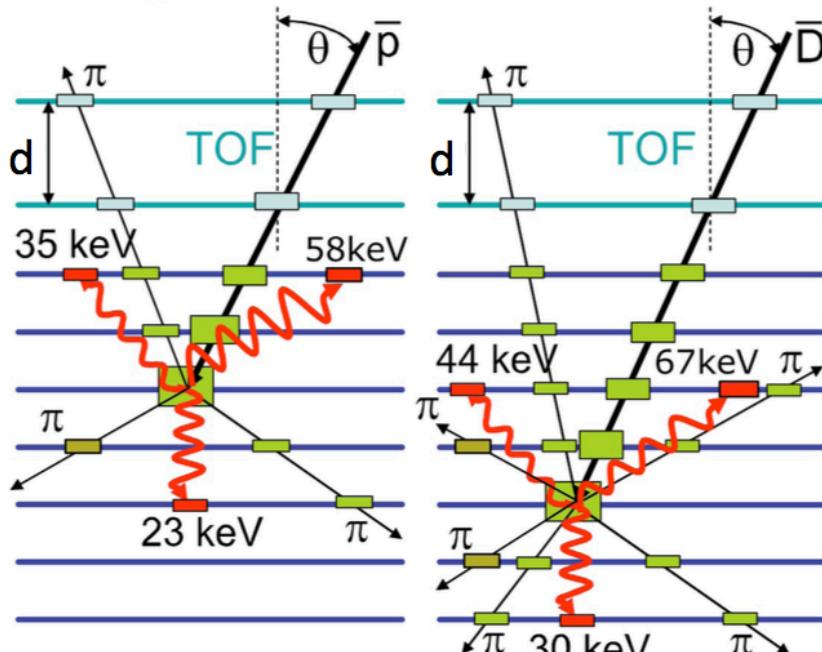
Low noise segmented Si(Li) detectors are used to reconstruct the event topology and identify the characteristics X-Ray
