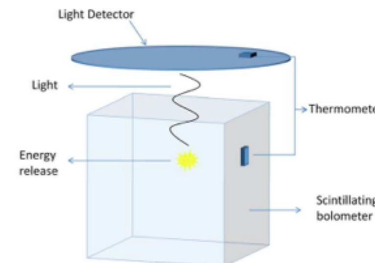
Requires ~20 eV resolution for >99.9%  $\alpha$  rejection @ >90% signal efficiency
