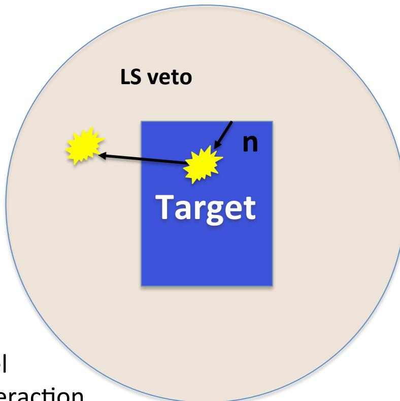
A radiogenic neutron from the cryostat steel or PMTs makes an interaction in target (WIMP-like) and later is captured in the LS veto. This type of event is rejected.
