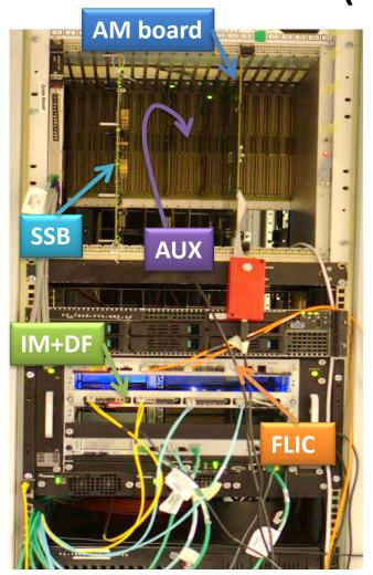
Communication and data flow test of few sets of all kind of boards using pseudo data are ongoing at Lab4.
