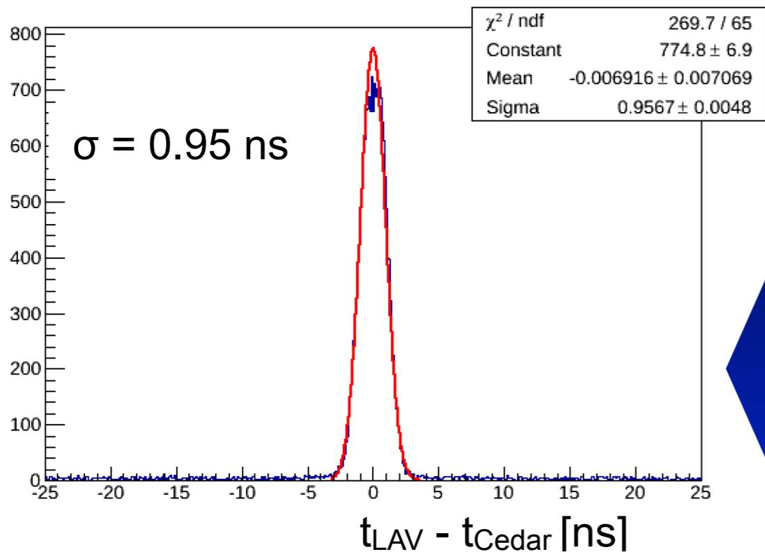
Time alignment after slewing correction
