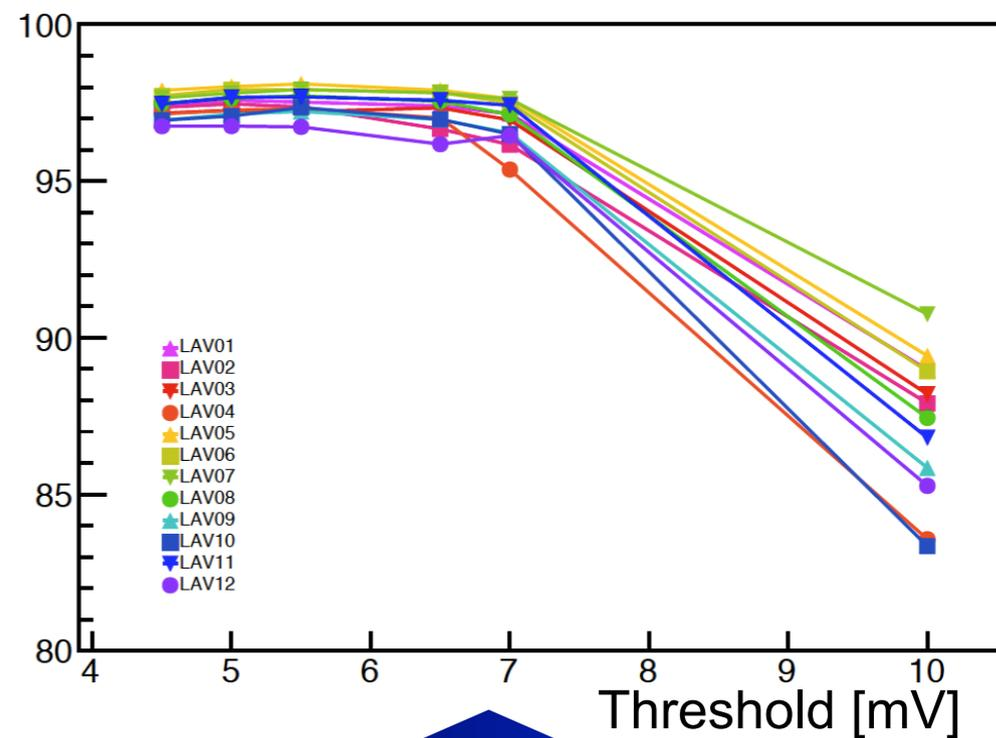
Muon efficiency vs threshold
