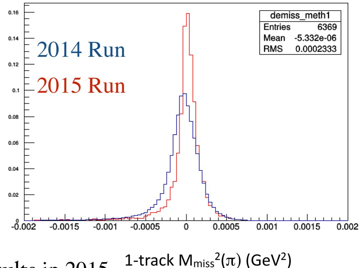
The K tracking system information and the full  $\pi$  spectrometer installation strongly improved the results in 2015
