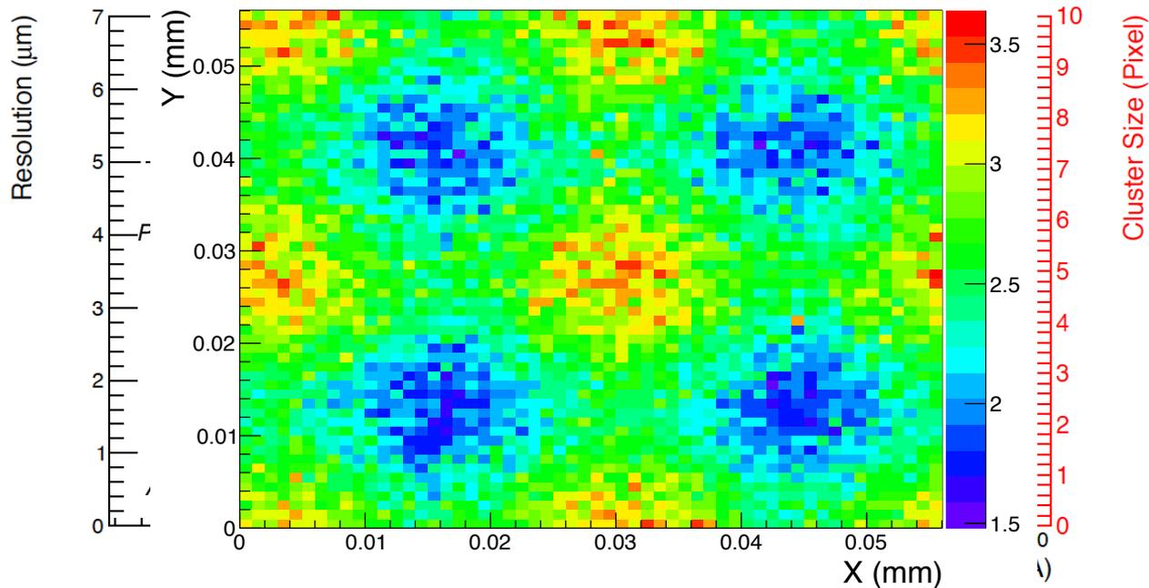
Space point resolution (including tracking error  $\sim 3 \mu\text{m}$ )  $< 5 \mu\text{m}$
