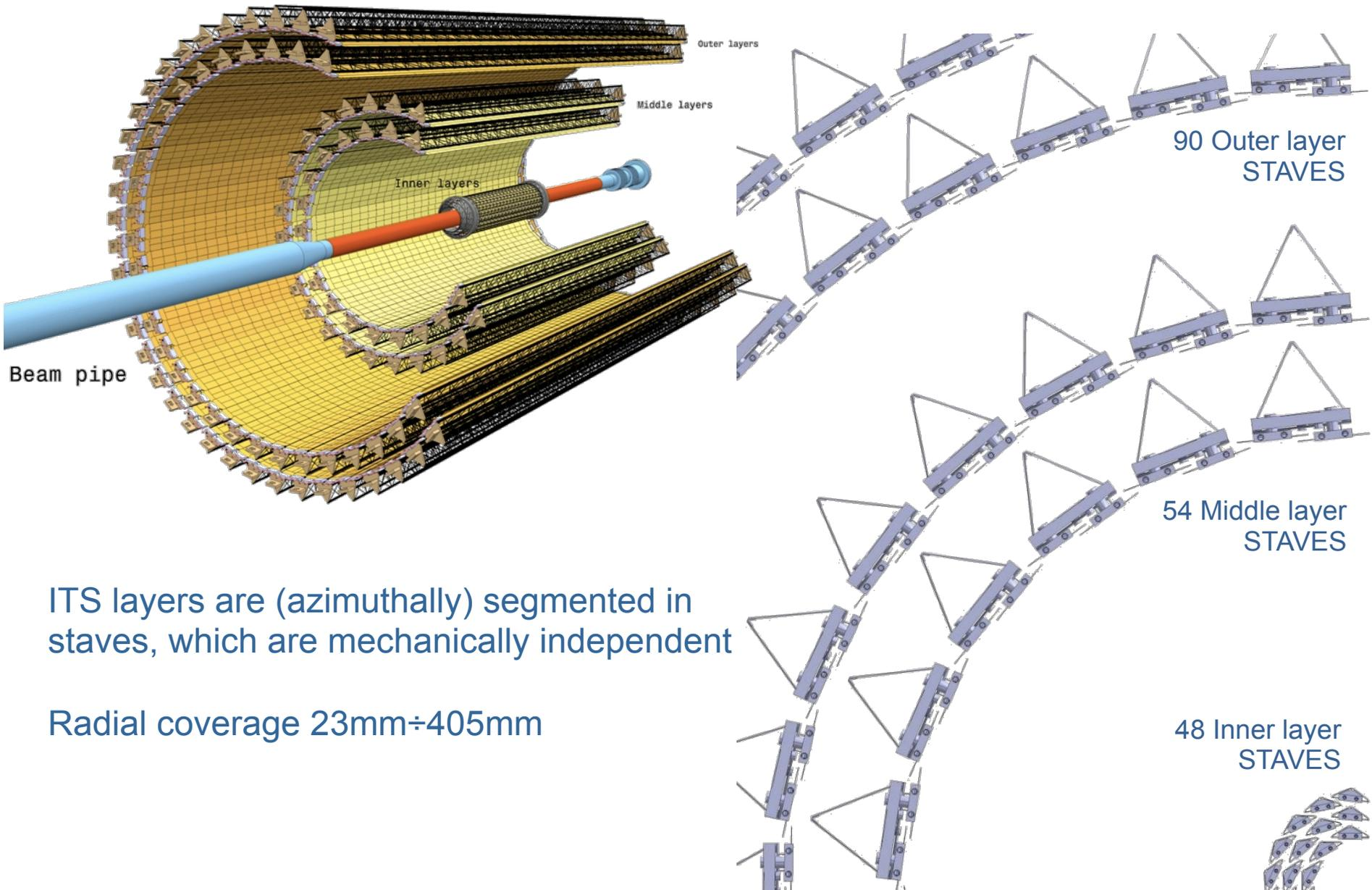
ITS layers are (azimuthally) segmented in staves, which are mechanically independent
