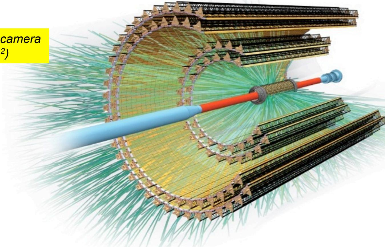
7-layer barrel geometry based on MAPS
