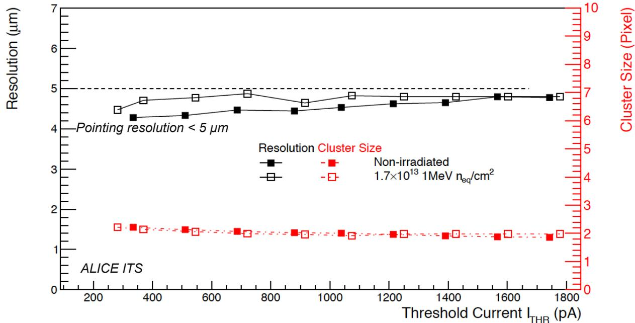
Space point resolution (including tracking error  $\sim 3 \mu\text{m}$ )  $< 5 \mu\text{m}$
