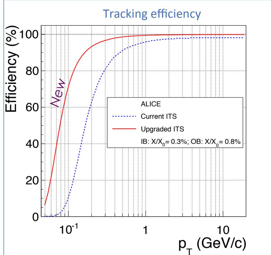
Fundamental improvement of the resolution (left) and tracking efficiency (right) from the old to the new ITS
