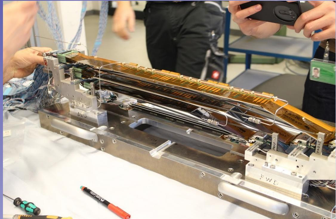
Test the integrated PXD-SVD system. This includes ROI (region of interest) extrapolation from the SVD tracker to the PXD, which is needed to reduce the *large data volume*.
