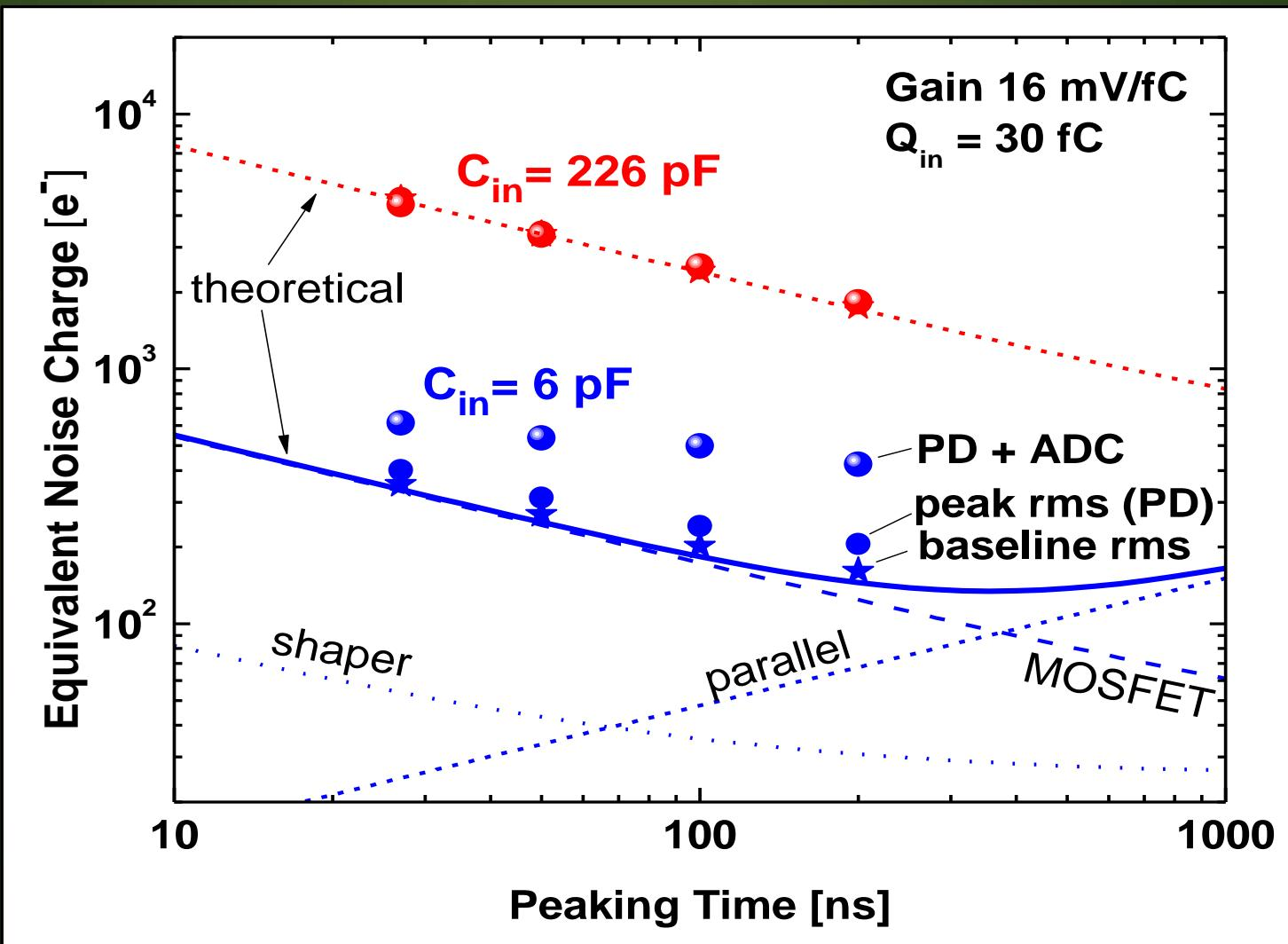
**ENC  $\sim 4,7k \text{ e}^-$  (0.75 fC) at 25 ns, 226 pF ( $\sim 5.6k$  at 0.5 mV/fC)**
