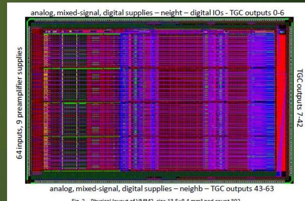
Fig. 2 – Physical layout of VMM2, size 13.5x8.4 mm<sup>2</sup> pad count 392.
