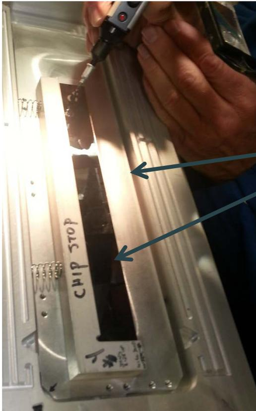
Precision vacuum chuck fixtures to **position sensors by hand**
