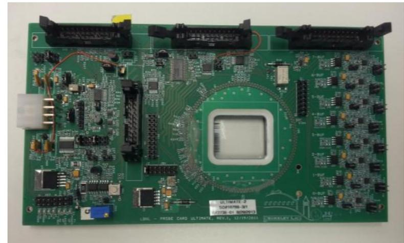
*Probe card with readout electronics*
