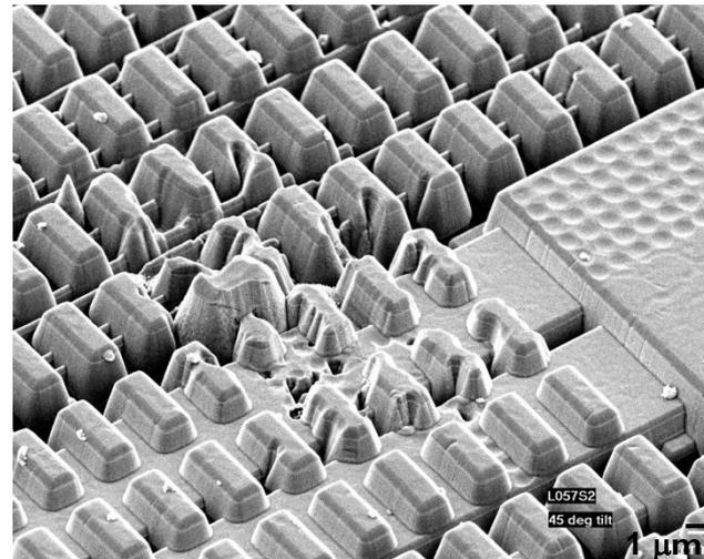
*Pixel sensor layers deconstructed (plasma etching technique) and viewed with SEM.*
