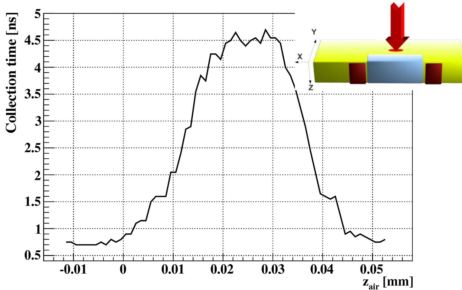
Collection time of signals shows implant depth~100  $\mu\text{m}$
