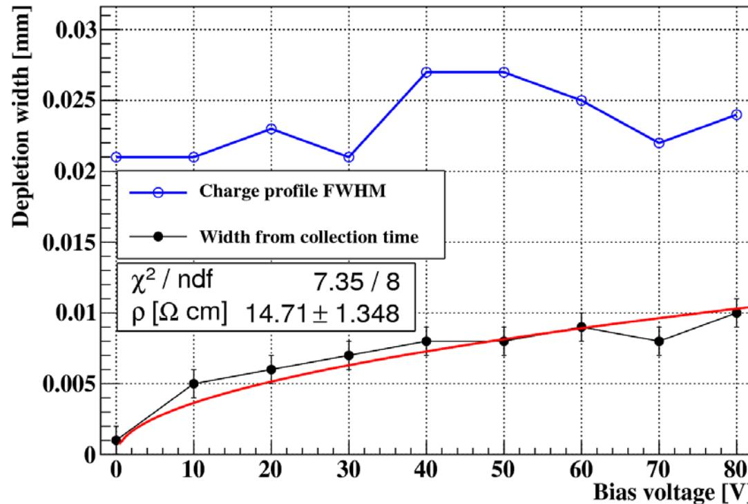
$$w_p [\mu\text{m}] = 0.3 \sqrt{\rho [\Omega \text{ cm}]} V$$
