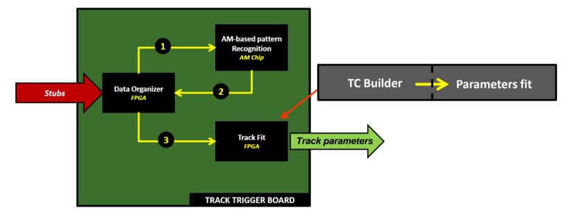
$\rightarrow$  The TC Builder proceeds to a **3D clustering** of the stubs **pattern per pattern**
