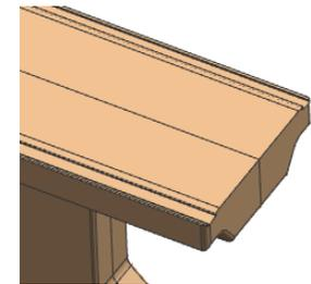
Longitudinal position of the groove and detail on the undercut region
