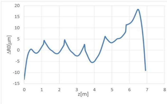
Average aperture perturbation in the case  $T_1=15^\circ\text{C}$ ,  $T_2=20^\circ\text{C}$ . The associated frequency shift is equal to 7 kHz and a voltage perturbation  $|\Delta V(z)/V(z)| < 0.005$ , to be compared with the maximum admissible value of 0.03, as for beam dynamics specifications.
