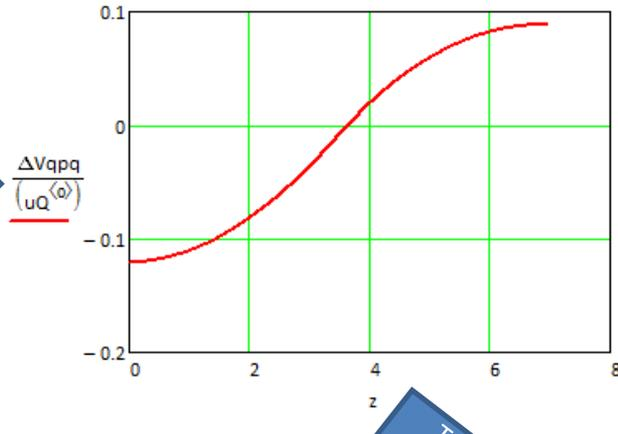
The effect is a  $\Delta V/V = \pm 10\%$  voltage variation and a frequency shift of -280 kHz
