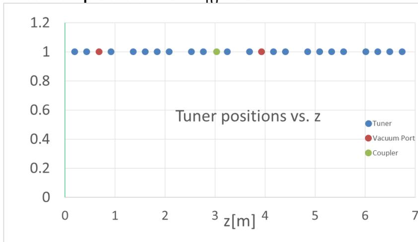
The amount of extra power  $\Delta P$  dissipated by the tuners, is  $\Delta P = (R_s/2)H^2 2\pi a N_T h_{t\max}$ ,  $R_s$  = surface resistance,  $H$  = magnetic field in the tuner location. In our case  $\Delta P/P_0 = 0.08$
