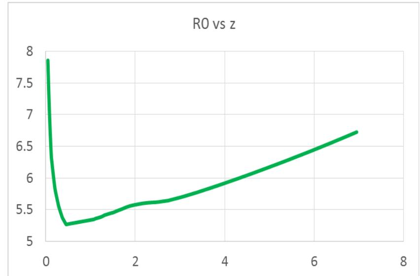
In order to implement  $V(z)$  all sections are designed with same constant  $TE_{21}$  cut-off frequency  $f_c=79.5 \text{ MHz}$  (see slides on the tuning) ; then by properly shaping the vane undercuts at the Low and High Energy Ends of the RFQ the desired voltage slope is obtained.
