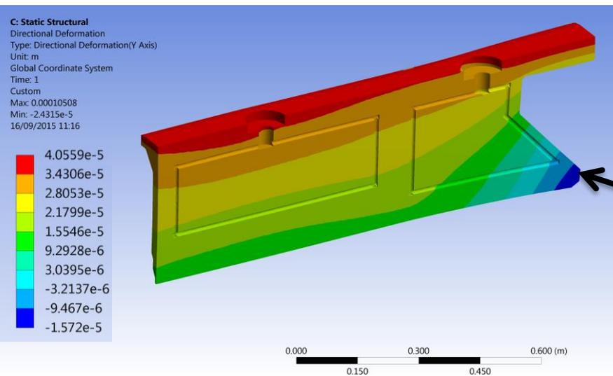
Maximum tip displacement 15  $\mu\text{m}$
