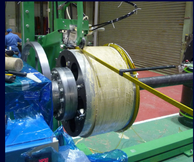
TS1a coil winding
