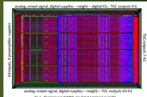
130nm 1.2V 8-metal CMOS technology from IBM
