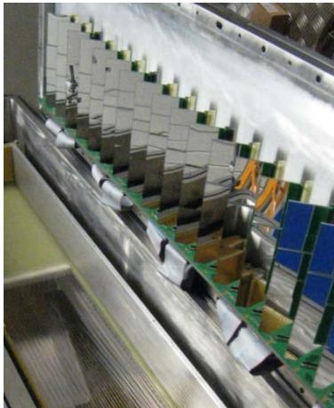
To wall of **2500 SiC-SiC pad telescopes**
