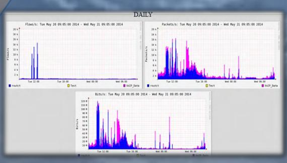
The nfdump tools collects and process netflow data on the command line. NfSen is a graphical web based front end for the nfdump netflow tools. It allows you to display your netflow data, easily navigate through the netflow data, process the netflow data within the specified time span, set alerts, etc.
