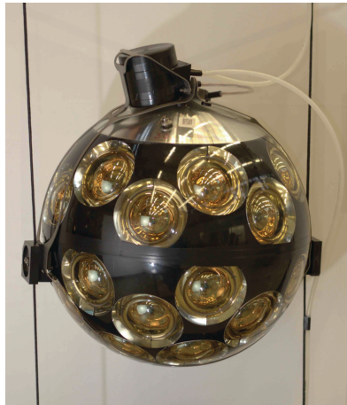
Figure 1. Picture of a DOM. The external collar, the break out box of the VEOC (Vertical Electrical-Optical Cable) backbone cable and the two parallel ropes of the detection unit are visible.
