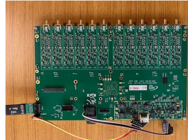
ID 12-channel front-end board
