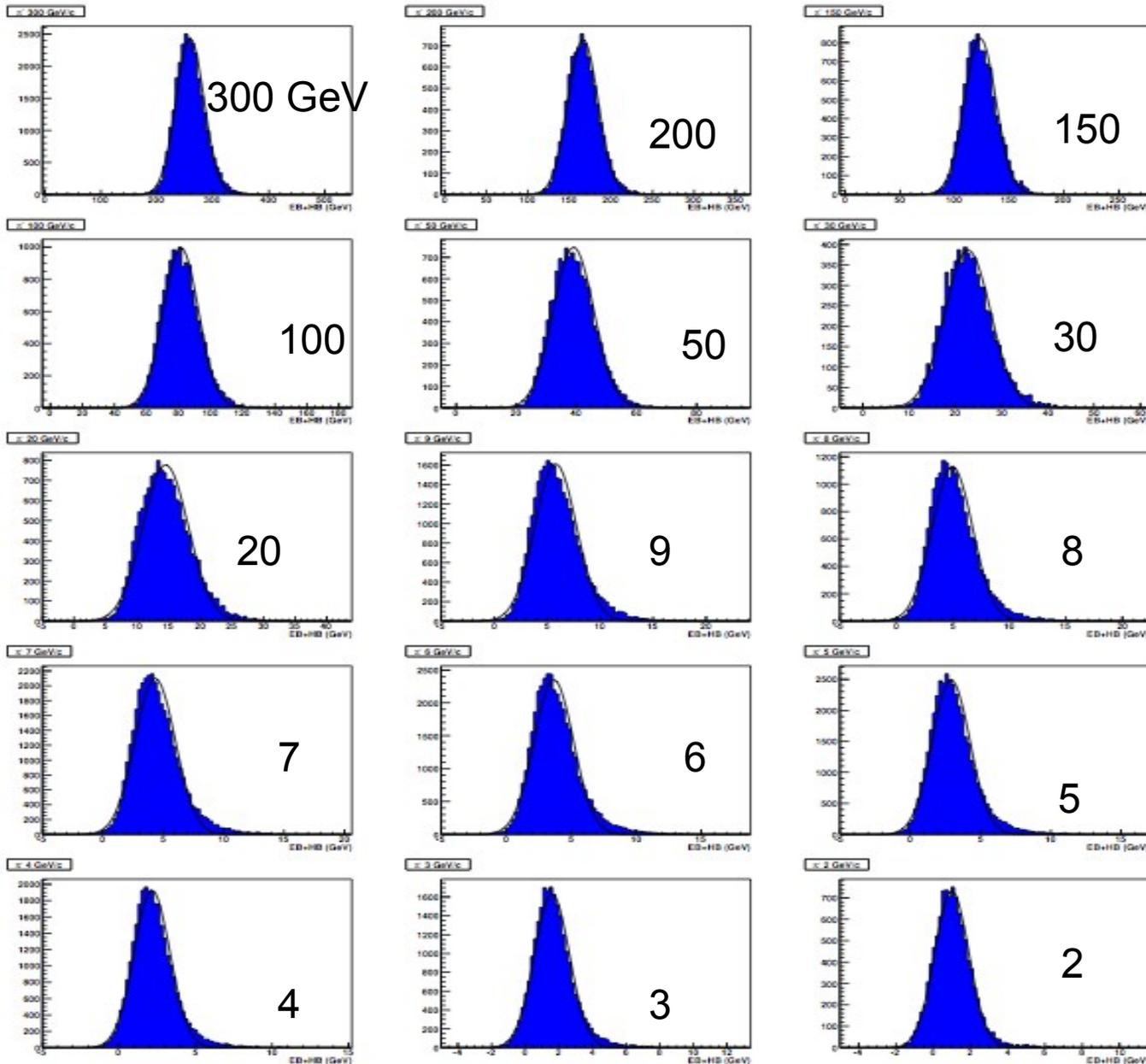
Without the noise cuts, the distributions are gaussian down to 2 GeV/c.
