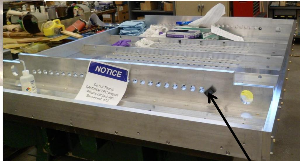
Holes for electronic-card cooling lines
