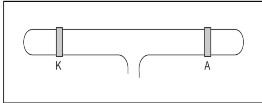
Fig. 3b  $p = 40$  mbar: small luminous cone in front of the cathode
