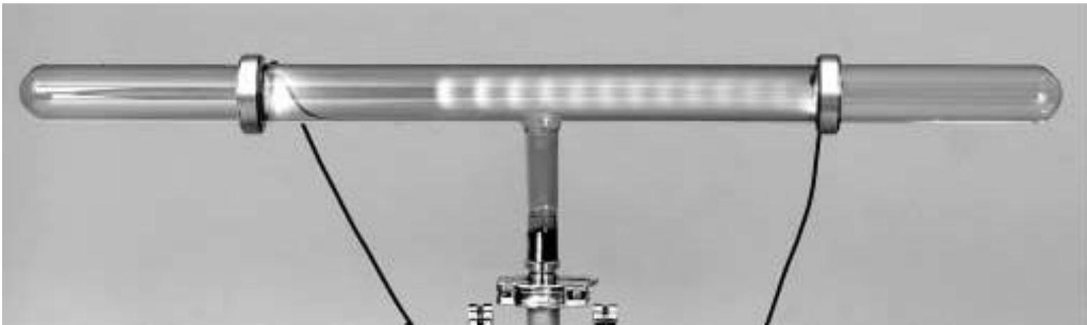
Fig. 3a  $p = 1013$  mbar: no discharge occurs ( $U = 5.0$  kV)
