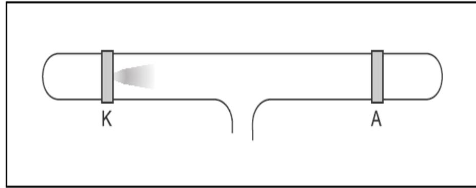
Fig. 3c  $p = 7$  mbar: the streamer becomes thicker (positive column), small luminous spot at the cathode, small dark space in front of the cathode ( $U = 1.1$  kV)
