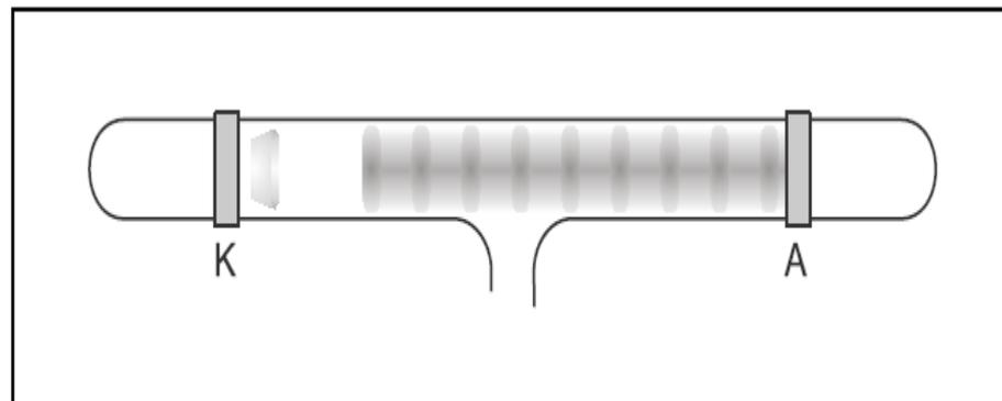
Fig. 3g  $p = 0.1$  mbar: dark space widens; layers in the positive column become mushroom shaped ( $U = 0.8$  kV)
