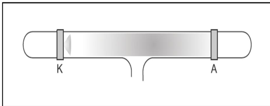
Fig. 3e  $p = 0.35$  mbar: positive column loses colour, and bright and dark zones emerge ( $U = 0.6$  kV)
