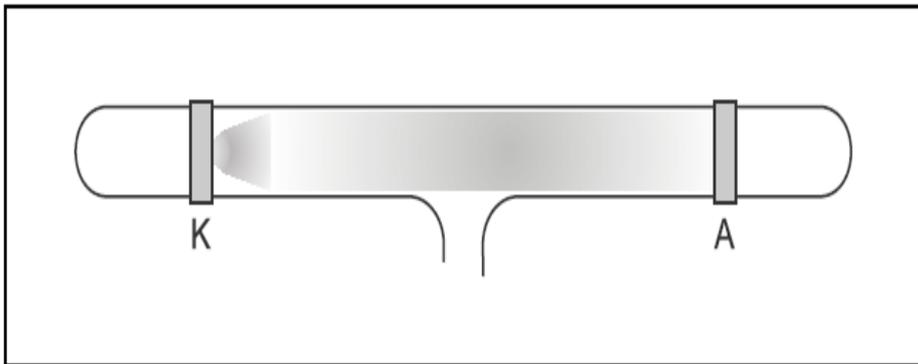
Fig. 3i  $p = 0.035$  mbar: glow light in front of the cathode disappears; in front of the anode fluorescence arises, and behind the cathode there is a luminous effect ( $U = 5.0$  kV)
