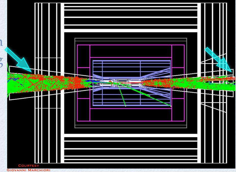
A very thick (~ 10 cm) tungsten shielding is needed to contain electromagnetic showers: 2 x ~300 k€
