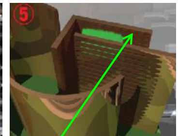
multiplication by n dynodes and signal on the anode
