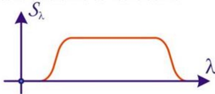
Because **thermal detectors** rely on only the amount of heat energy delivered, their response is independent of wavelength.
