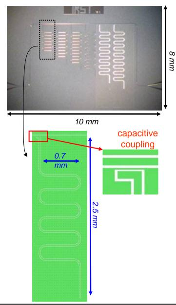
Material: Aluminium 6 resonators of varying length
