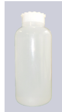
water phantom (radius = 6 cm) containing NaCl 0.1M ( \sigma = 1 \text{ S/m} )
