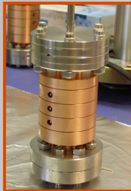
Copper model and longitudinal electric field profile of the operating mode
