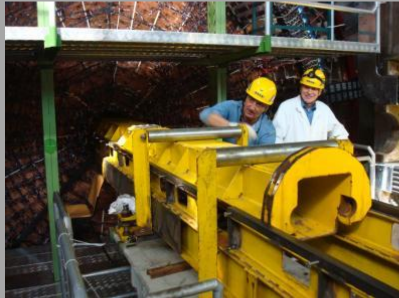
Insertion of the beam guide in the Kloe DC;
