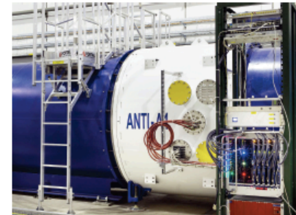
A Large Angle Veto detector in place in the NA62 decay volume.
