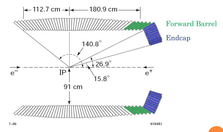
Figure 3-11. The EMC layout: Side view showing dimensions (in mm) of the calorimeter barrel and forward endcap.
