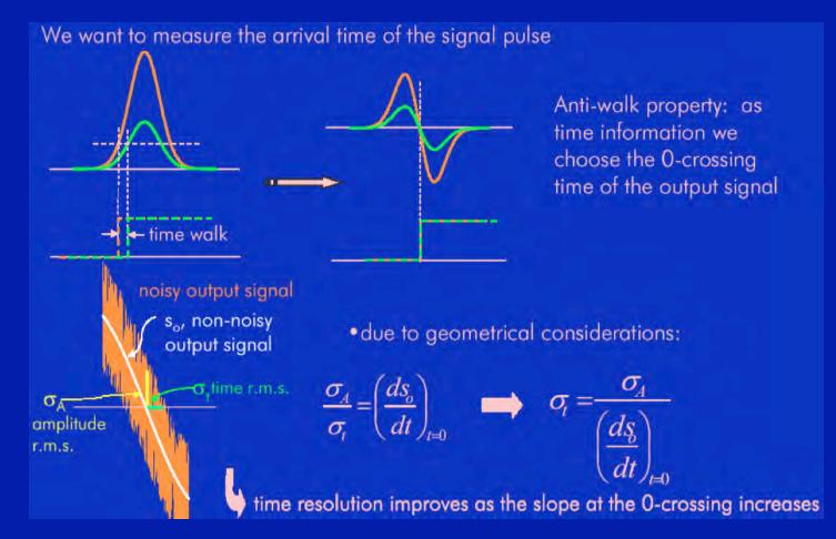
• The amplifier speed is important, but so is the amplifier noise!
