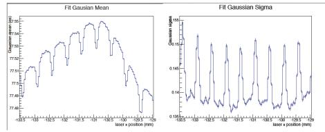
Fit to Box Convoluted with a Gaussian Gaussian Sigma for Internal Pads ~450  $\mu\text{m}$  For Edge Pads, ~540  $\mu\text{m}$  (4 $\sigma$  beam spot ~50  $\mu\text{m}$ )
