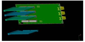
4 analog boards with the SCATS CRT ( bottom view)
