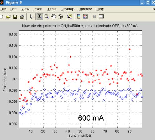
DAFNE e+ beam, 100 bunches, spaced by 2.7ns with 20 buckets gap
