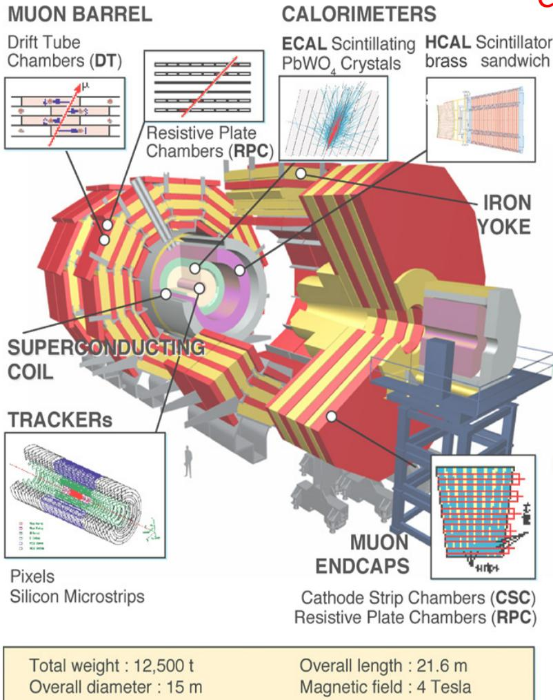
CMS design choice: optimize performance for muon / track momentum resolution (and electromagnetic energy resolution)
