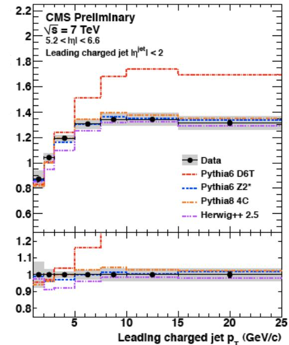
Energy deposited in CASTOR ( $5.2 < |\eta| < 6.6$ ) for events with a charged particle jet in the central pseudorapidity region  $|\eta_{\text{jet}}| < 2$ , as a function of charged particle jet transverse momentum  $p_T$  (normalized to the average energy in inclusive events)
