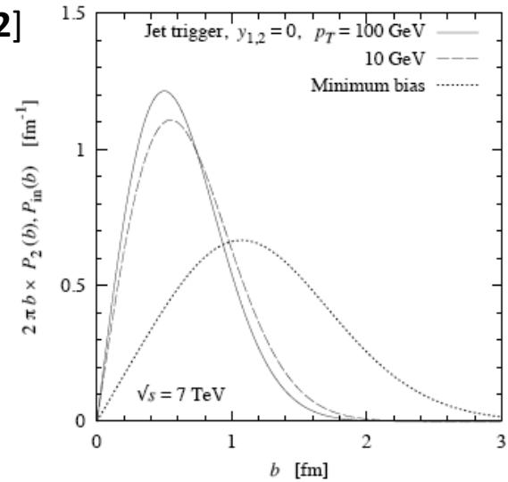
Impact parameter distributions of inelastic pp collisions at  $\sqrt{s} = 7$  TeV. Solid (dashed) line: Distribution of events with a dijet trigger at zero rapidity,  $y_{1,2} = 0$ , c, for  $p_T = 100$  (10) GeV. Dotted line: Distribution of minimum-bias inelastic events (which includes diffraction).
