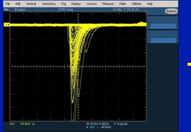
(Single photoelectrons in SLAC scanning setup)
