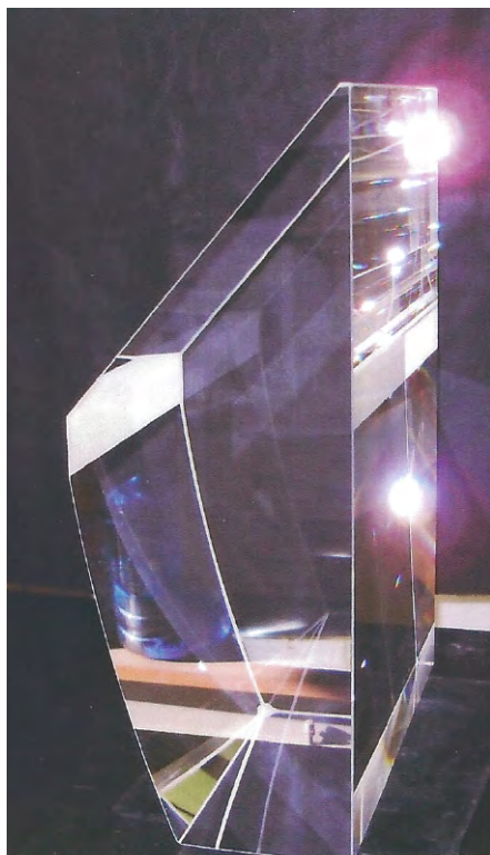
(a) FBLOCK after polishing but before plating.
