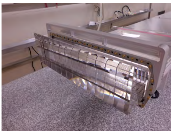
(b) Detailed view of the New Wedge and the bar box window.
