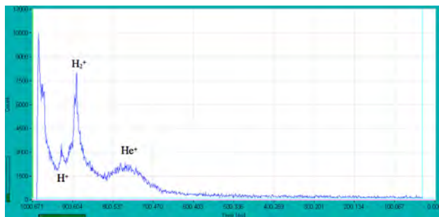
Figure 1.50: A time spectrum of after pulses showing H^+ , H_2^+ and He^+ contamination [26].
