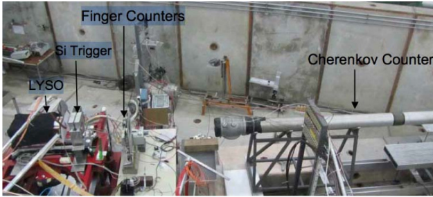
Figure 9.30: Schematic view of the test beam setup used at CERN.
