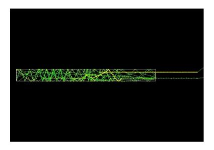
Simulation of a plastic bar using Geant4, with two fibers..(I. leon)
