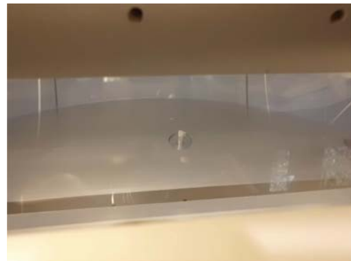
(b) OPAL diffuser used to spray laser photons into the FBLOCK.
