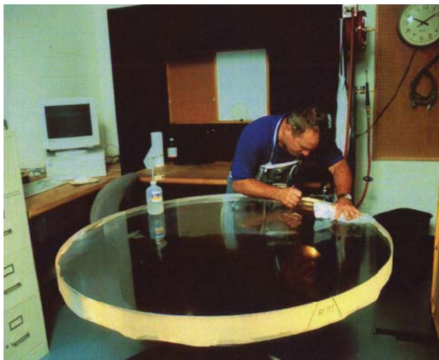
Figure 1.37: An example of the fused silica 7980 material in the form of a 60 inch dia. boule made by Corning.
