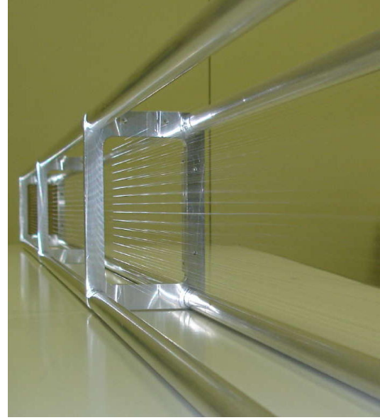
Figure 7.5: Prototype 2: detail of the strung wires.
