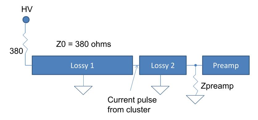
Example: 50,000 electrons in 1 nanosecond =  $8 \mu A$  => 1.52 millivolts in 380/2 ohms
