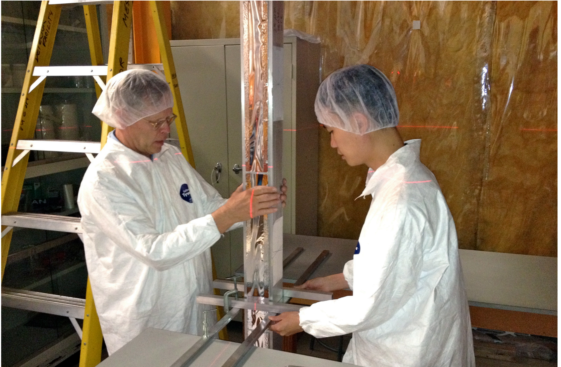
Wayne and Rocky restringing the prototype with 30\mu sense wire
