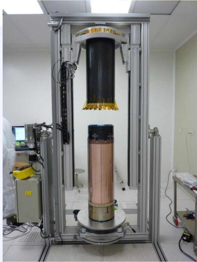
Everything is aligned with an axial precision of 0.1mm/1.5m
