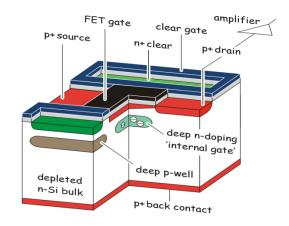
DEPFET - monolithic silicon active pixel sensors which do not require additional support or cooling structures in the active region of the detector. Spatial point resolutions below 10 µm are expected.
