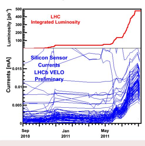
The leakage currents of all 88 sensors plotted against time. Currents are measured at -8 °C without beam. The LHC integrated luminosity is also shown as a guide to the fluence.
