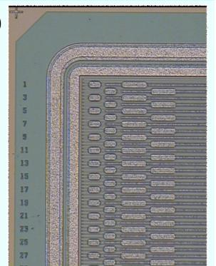
Detail of a corner of the telescope strip detector.
