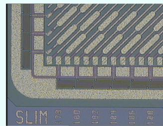
Detail of a corner of the striplet detector.
