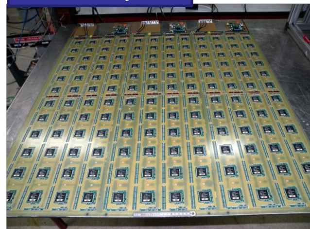
1m 2 equipped with 144 MICROROC
