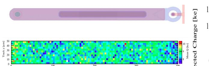
Mean collected charge as a function of the track impact point for a module irradiated up to  $5 \times 10^{15} n_{eq} \text{ cm}^{-2}$  and biased at 600 V.
