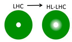
Qualitative illustration of the expected degradation of FCal1 in r/phi with luminosity increasing from LHC to HL-LHC
